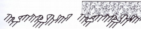
FIGURE 4.4 Time, choice of a suitable viscosity and curing time enable the flow of a liquid adhesive into the interstices of a substrate and the flow of air away from the pores in the interface. This increases mechanical interlocking of the adhesive with the adherend, the difficulty of reversing the joint and removing the adhesive. Adapted from Pocius (2002).
