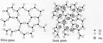
Figure 4.4 The arrangement of elements in glasses
